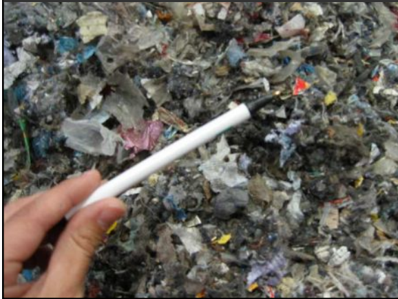
Indust. paper plastic, textile =>shredded on site
